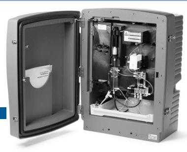
The Hach PHOSPHAX sc Phosphate Analyzer measures PO<sub>4</sub>-P concentrations as low as 0.05 mg/L and as high as 50 mg/L. And operation costs are low because it uses 50% less chemicals. This is no "black box" system—you get transparent, high-quality measurements for reliable values.
