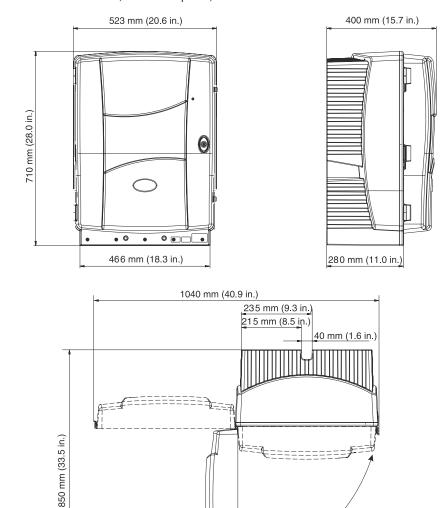
The Filterprobe sc should be installed at least 20 inches from the bottom and walls of the tank and must have at least four inches, but no more than 10 feet, of water above it.
